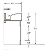
WT6 Profile Concealed waste trough with wall mounted taps. A choice of underframe or brackets.
