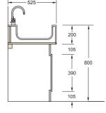
Maximum single Solid Surface washtrough length is 3000mm. Any stud framework is by site.
