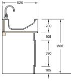
WT1 Thermo Profile Thermoformed trough with deck mounted taps. A choice of underframe or brackets.
