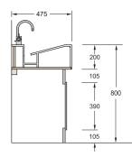
WT5 Profile Concealed waste trough with deck mounted taps. A choice of underframe or brackets.
