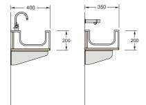
WT4 Thermo WT3 Thermo Slim Profile Slim Profile Slim thermoformed Slim thermoformed trough with deck trough with wall mounted taps. A mounted taps. A choice of brackets choice of brackets or underframe. or underframe.
